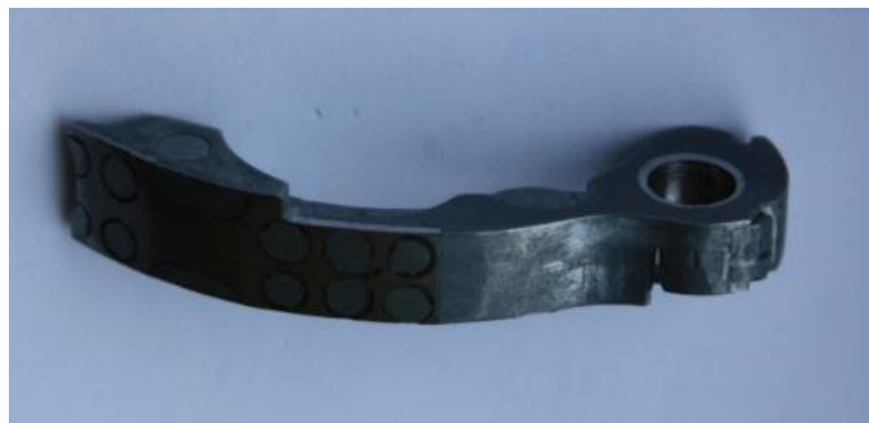
Figure 39: Die cast AISI D2-Zamak 5 inserted hammer. Neither deformation nor cracks were visible after hundreds of cycles.
