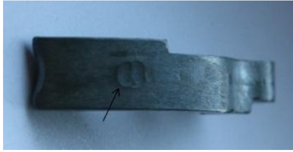
Figure 38: Operated monolithic (non-inserted) Zamak5 hammer. Despite perfect shots, inelastic deformation was occurred at the impact point.
