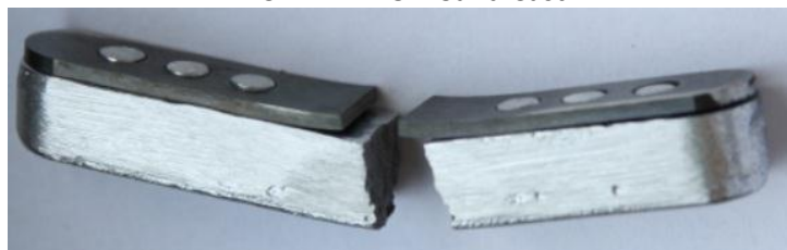
Figure 48: Broken Charpy impact test samples
