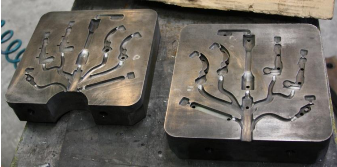
Figure 16: AISI 2344 Die casting molds used in experiments. Nitriding operation was held on whole casting surface to obtain hardened protection layer.
