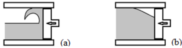
Figure 1: Entrapped air when plunger velocity is too fast (a), and too slow (b)
