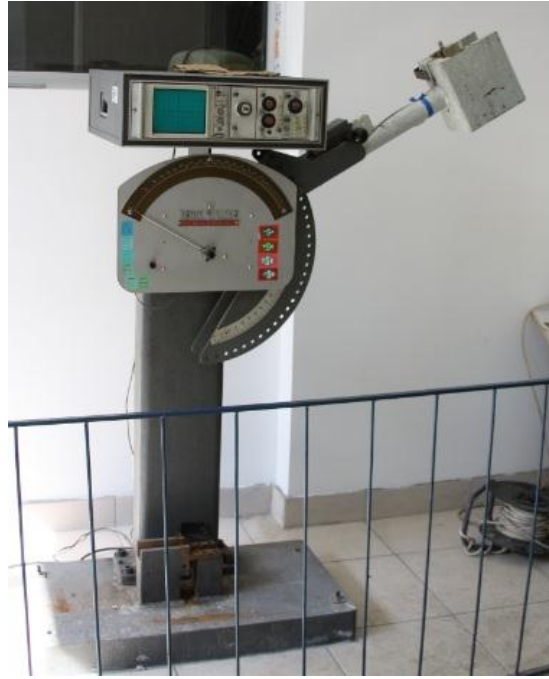
Figure 19: Charpy impact test equipment used in experiments
