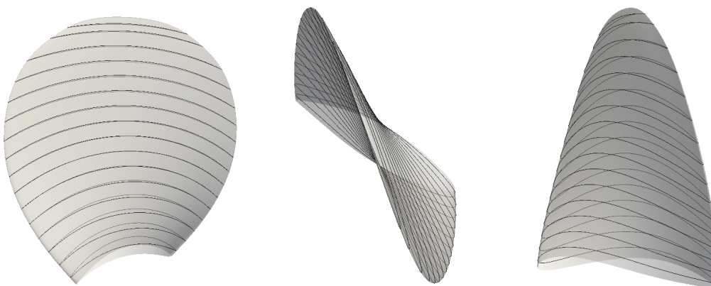
Figure 4.2 : Radial sections of DTMB 4119 propeller blade.
