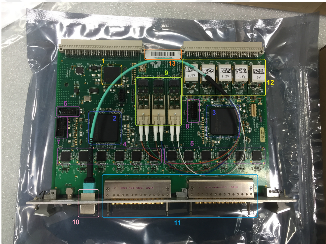
Figure 6.1. Front face of a QIE card with its components numbered as; 1: Bridge FPGA, 2: Top Igloo2 FPGA, 3: Bottom Igloo2 FPGA, 4: Top QIE10 Chips (Channels 7-12), 5: Bottom QIE10 Chips (Chan. 19-24), 6: Bridge FPGA programming port, 7: Top Igloo2 programming port, 8: Bottom Igloo2 programming port, 9: VTTx, 10: MTP connector, 11: Winchester connectors (PMT inputs), 12: DC-DC converters. 13: CMS identification sticker
