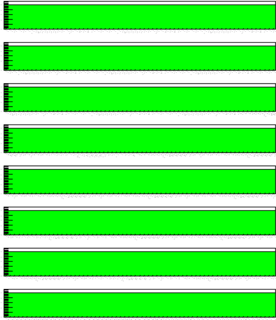
Figure 7.4. Result of a successful register test. The first seven rows and left half of the bottom row show the status of the registers involving QIE chips. Right half of the bottom row represents the Igloo2 registers.
