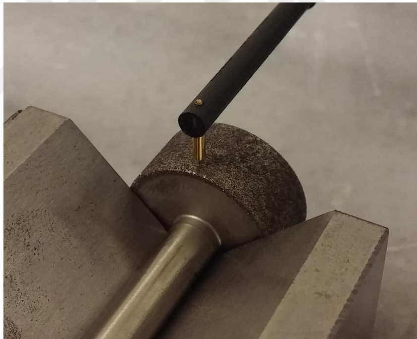
Figure 55- Surface Roughness of Electroplated CBN Grinding Wheel Measurement
