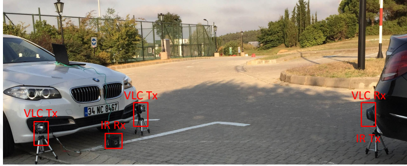
Figure 4.4: VLC and SecVLC Experimental Setup
