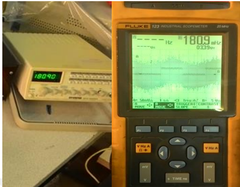
Figure 4. 13. The view of the zoomed oscilloscope screen with output signal with very low frequency value
