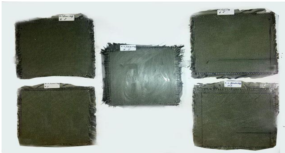
Figure 3.5 Examples of produced composite and hybrid composite plates
