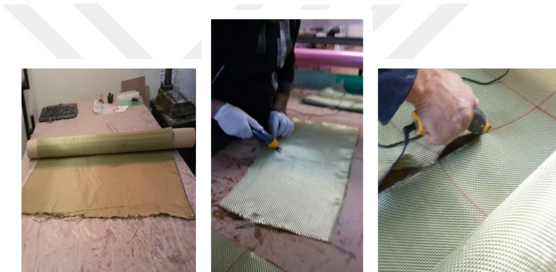
Figure 3.2. Cutting fibers by EC, (Kevlar / Carbon)
