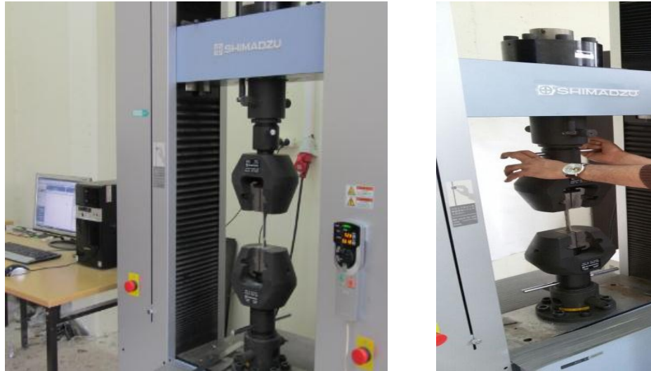
Figure 3.8 Test set-up Shimadzu AG-X series testing machine
