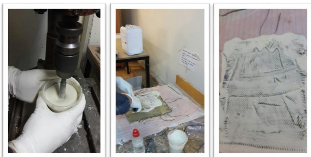
Figure 3.3 Mixing and application of Nano-clay and epoxy resin
