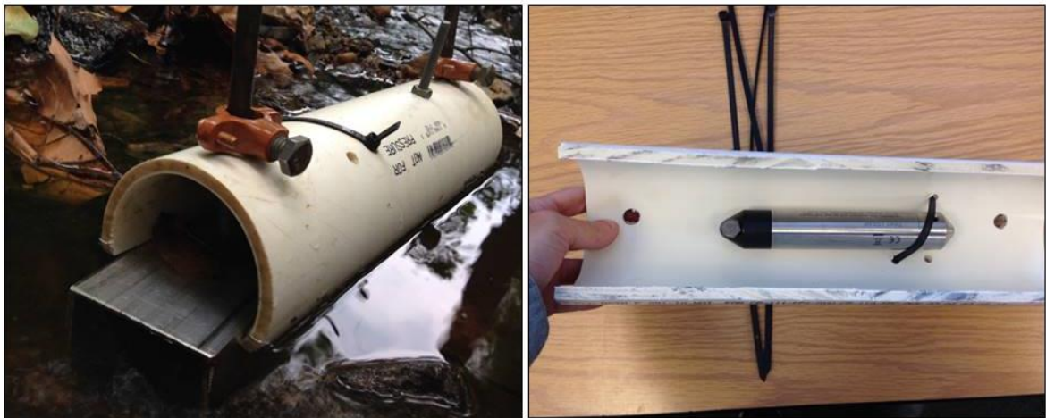
Figure 8.2. Pressure Recording Instruments (Water Level Logger) Used by the Author in a Watershed Project.
