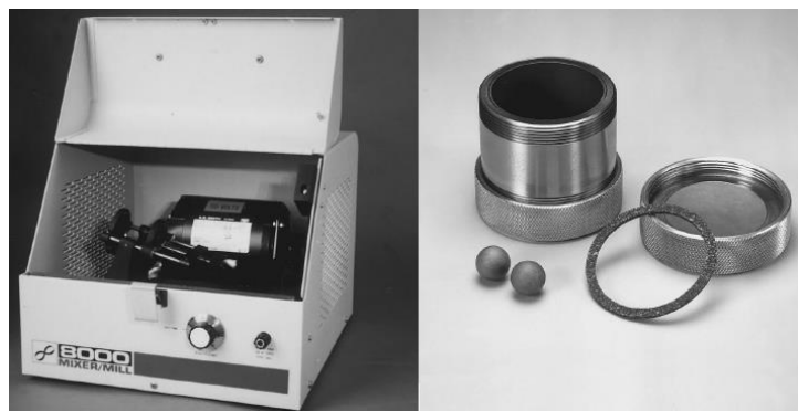
Figure 2.8 : SPEX 8000 mixer/mill in the assembled condition and Tungsten carbide vial set consisting of the vial, lid, gasket, and balls (El-eskandarany M.S.,2000).
