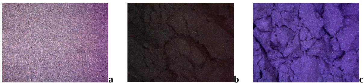
Figure 3.1 : stereomicroscope (SM) images of the raw materials: (a) W, (b) Ti, (c) LaB 6 .
