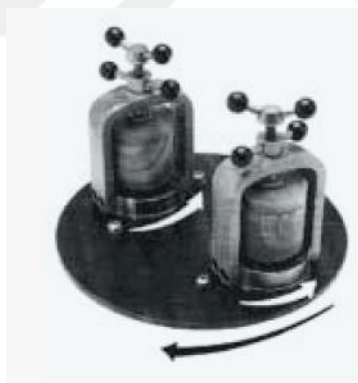
Figure 2.9 : Schematic view of planetary mills (El-eskandarany M.S.,2000).
