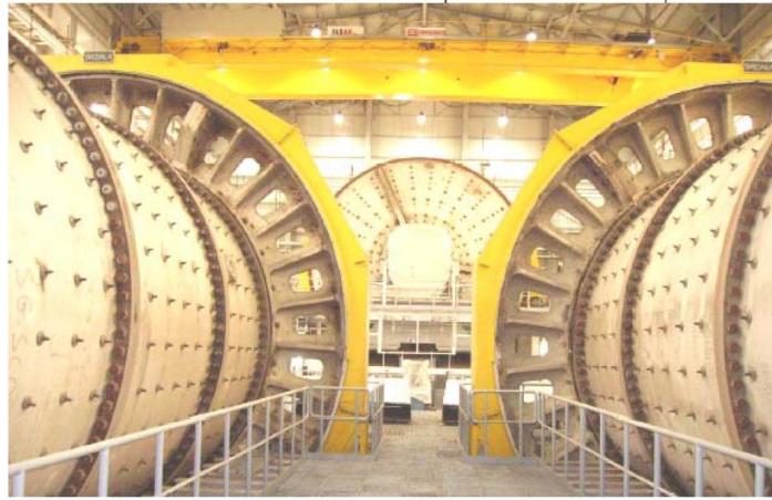
Figure 2.11 : Ball mills used in Iran copper concentration plant.
