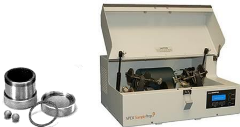
Figure 3.5 : WC vial and WC Balls and Spex™ Duo Mixer/Mill 8000D.
