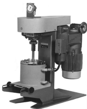
Figure 2.10 : Schematic view of attritor mills, (Surryanarayana, 2001).
