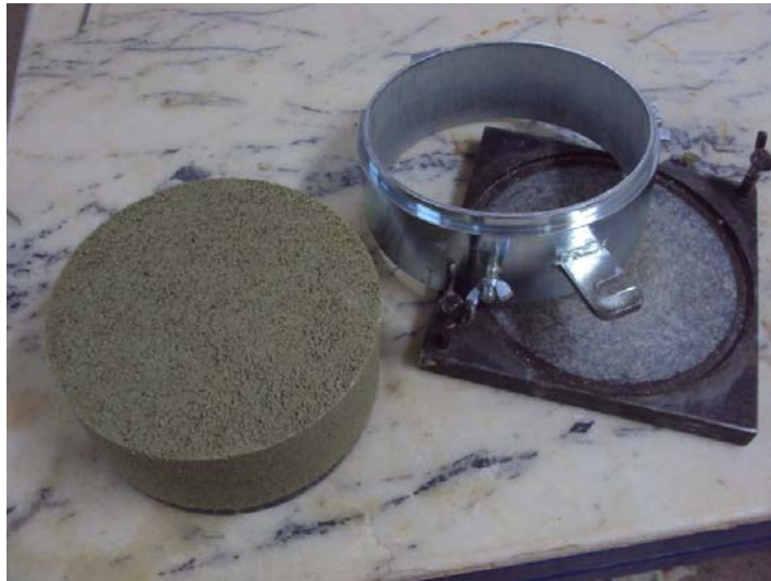
Figure 4.3 Compaction mold for hydraulic conductivity tests and compacted zeolite-bentonite mixture (ZBM).
