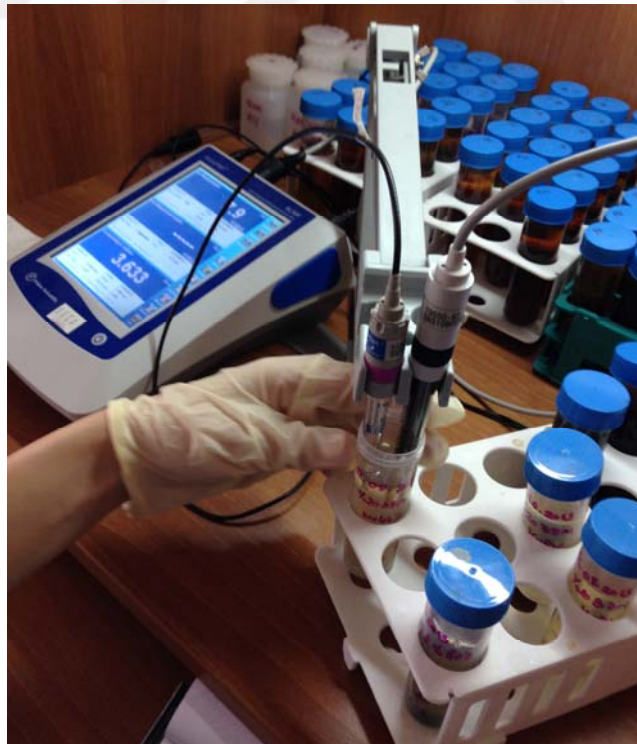
Figure 4.8 pH and Electrical Conductivity (EC) Meter and relevant probes that were used to control the chemical stability throughout the hydraulic conductivity tests.
