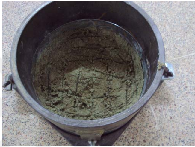
Figure 4.4 Scratching of the surface after compacting the first layer.
