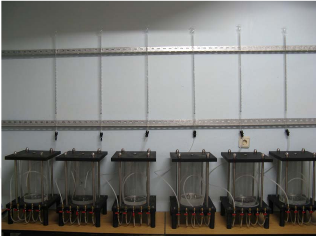
Figure 3.4 Installed ready-to-use flexible wall permeameters.
