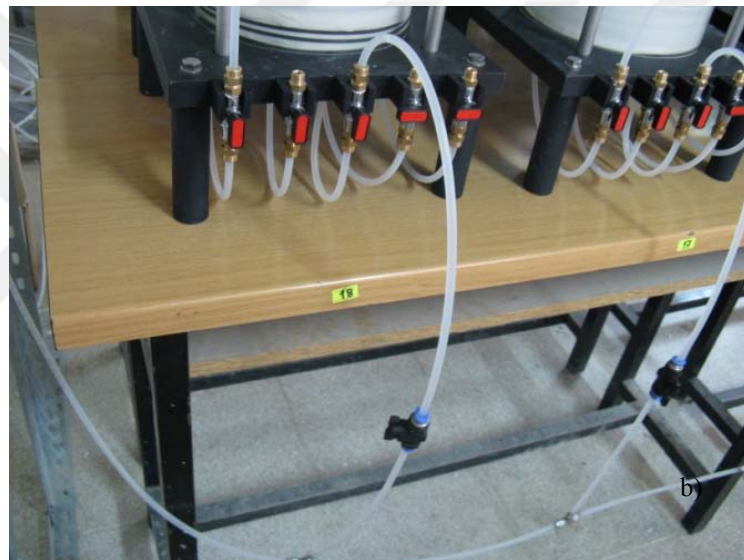
Figure3.1 Experimental setup in the Soils Lab.: a) pressure panel, b) internal connections between the panel and the permeameters.
