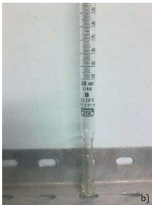
Figure 3.2 Experimental setup in the Soils Lab: a) the metal frame and burettes, b) details of a burette and c) tubing and reductor mounted on the burette.
