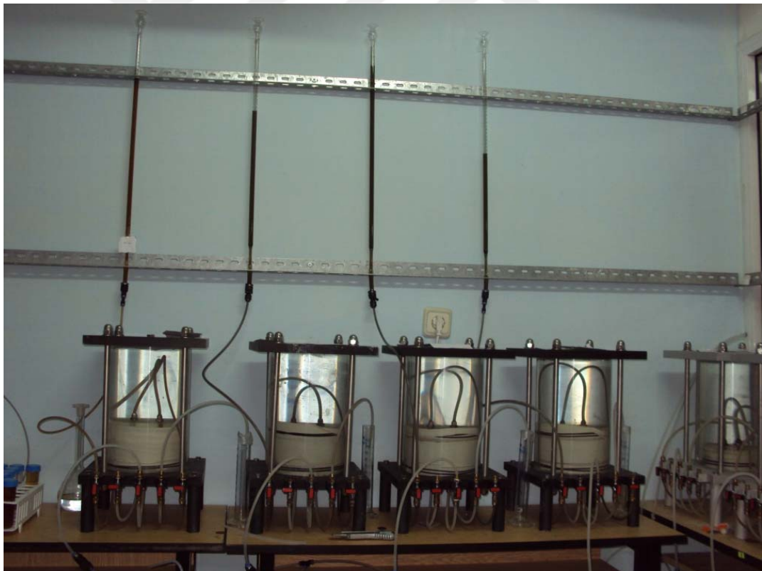
Figure 4.7 Overview of the hydraulic conductivity system and the test samples.
