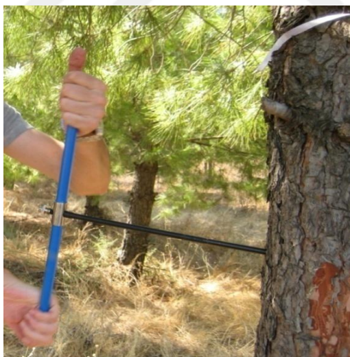
Figure 3.10 Collection of tree ring samples by using increment borer
