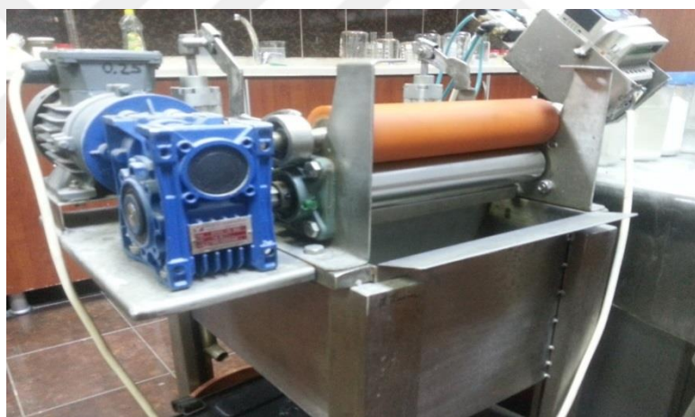
Figure 3.4. Laboratory type of kiss-roll machine
