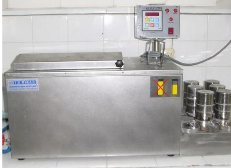
Figure 3.5. Laboratory type laundering machine
