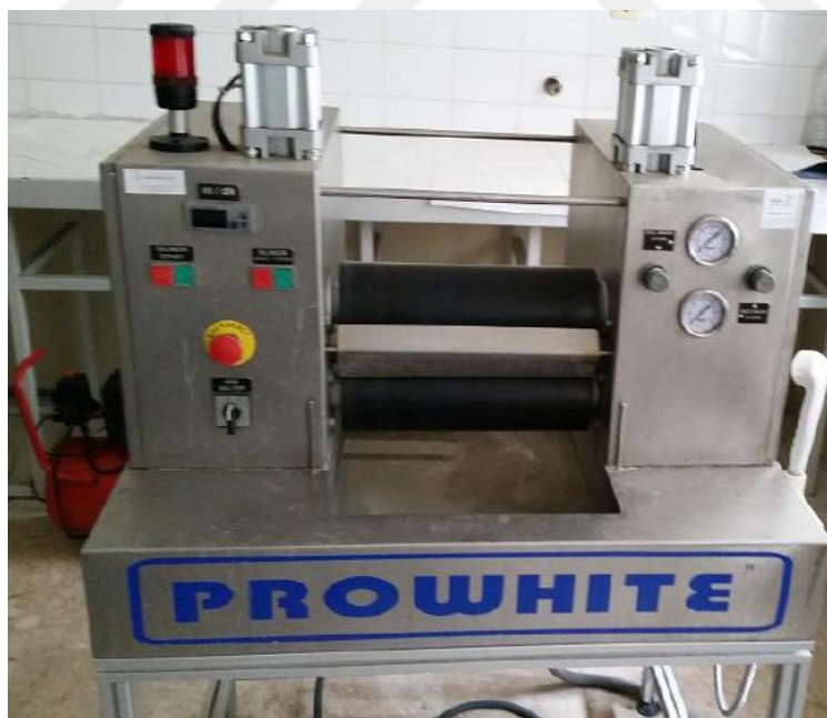
Figure 3.3. Laboratory Type Padding Machine
