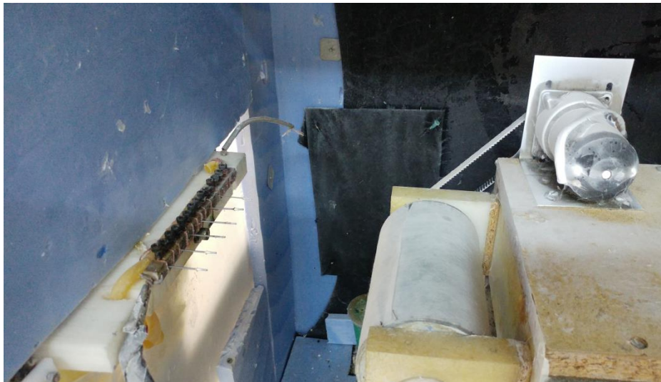
Figure 3.2. Needles and collector
