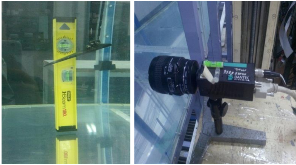
Fig.3.5. Experimental Setup with CCD camera for Calibration
