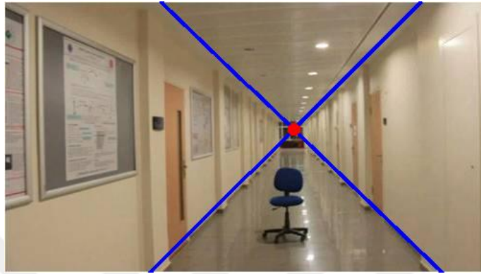
Figure 3.2. Determined geometrical cues of a background structure: vanishing point is marked by a red point and main lines are showed as blue lines
