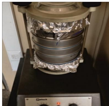
Figure 3.4.1 : Stack of sieve sets for sieve analysis from ITU-General Geology Laboratory.
