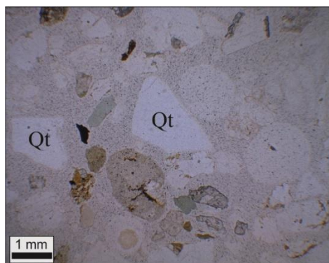
Figure 4.1.3.4.2 : Photomicrograph of Maritsa River-Sample 1. (a) is under plane polarized light, (b) is view from cross-polarized light (XPL). Qt refers to quartz grain in the thin section.
