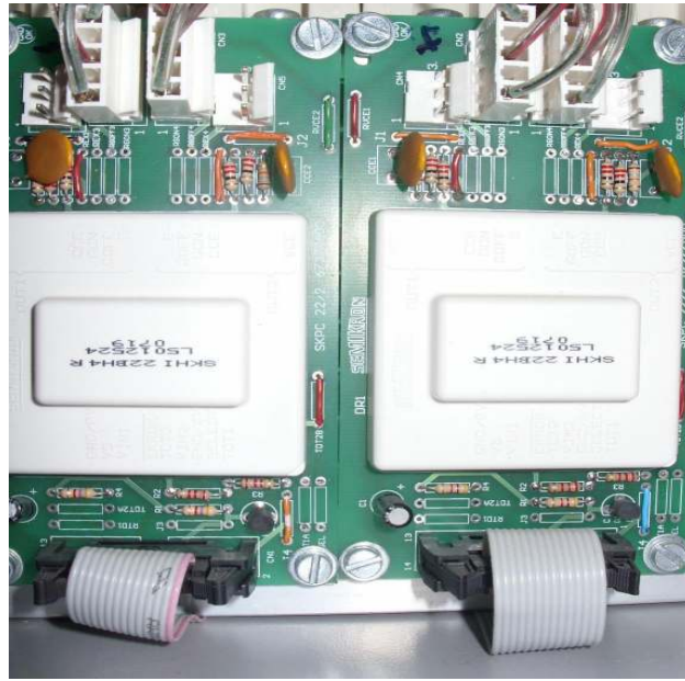
Figure 4.24. IGBT driver cards for one of h-bridge inverters
