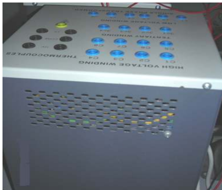
Figure 4.27. Single phase injection transformer
