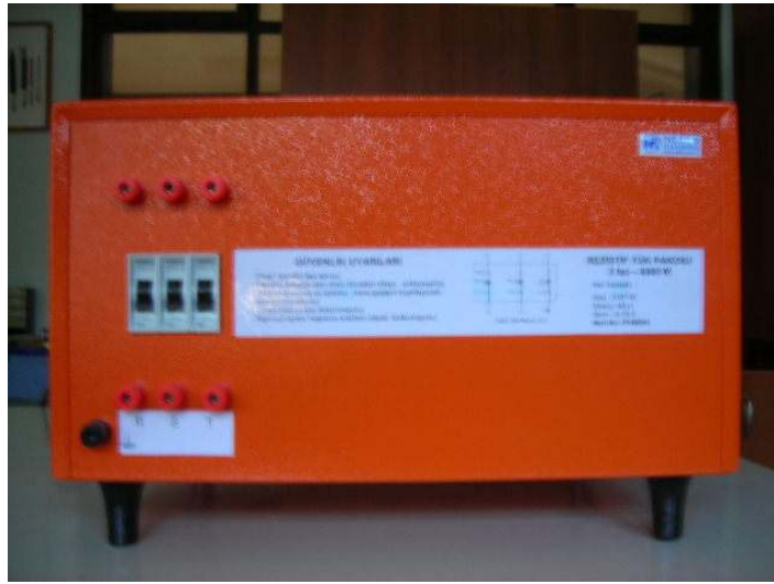
Figure 4.28. Three phase 3 kVA load
