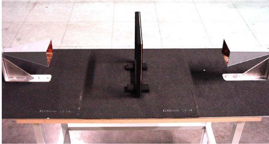
Figure 3.5: Free Space Dielectric Measurement Setup
