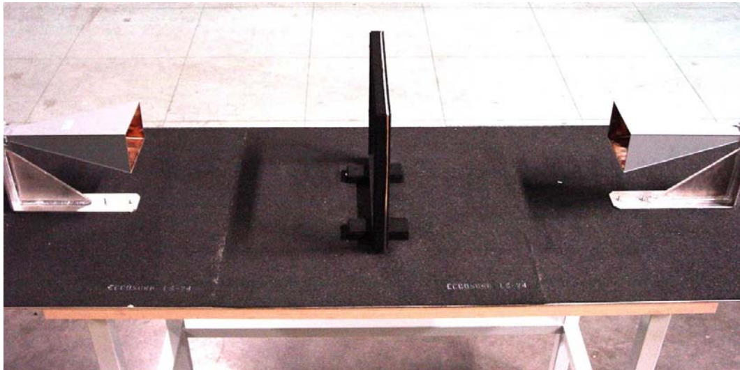
Figure 4.3: Free Space Transmission Measurement Setup
