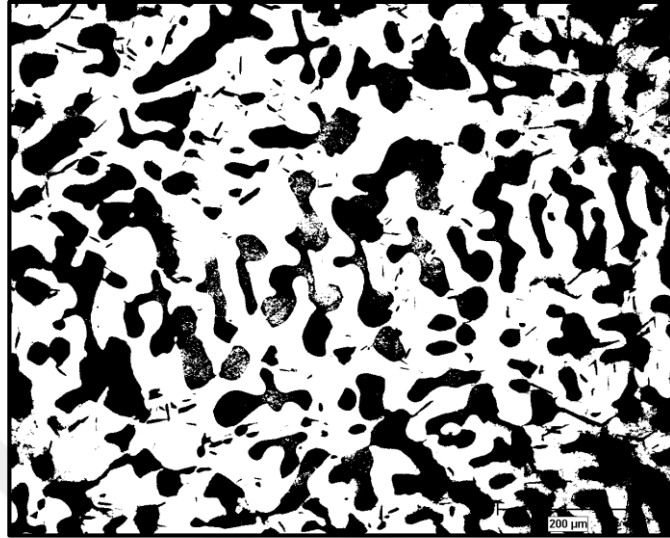
Figure 4.23 ImageJ phase analysis image of the sample ST-1150 / A-700-8 (Air cooled)
