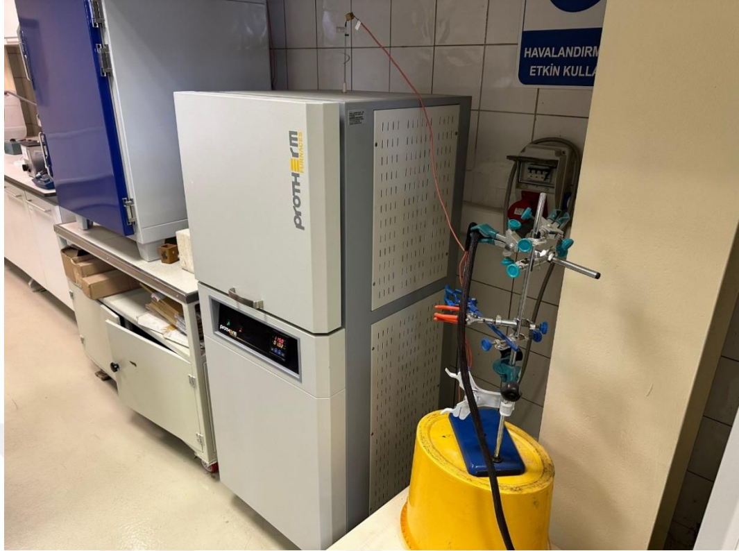
Figure 3.6 Protherm furnace and ORDEL thermocouple system
