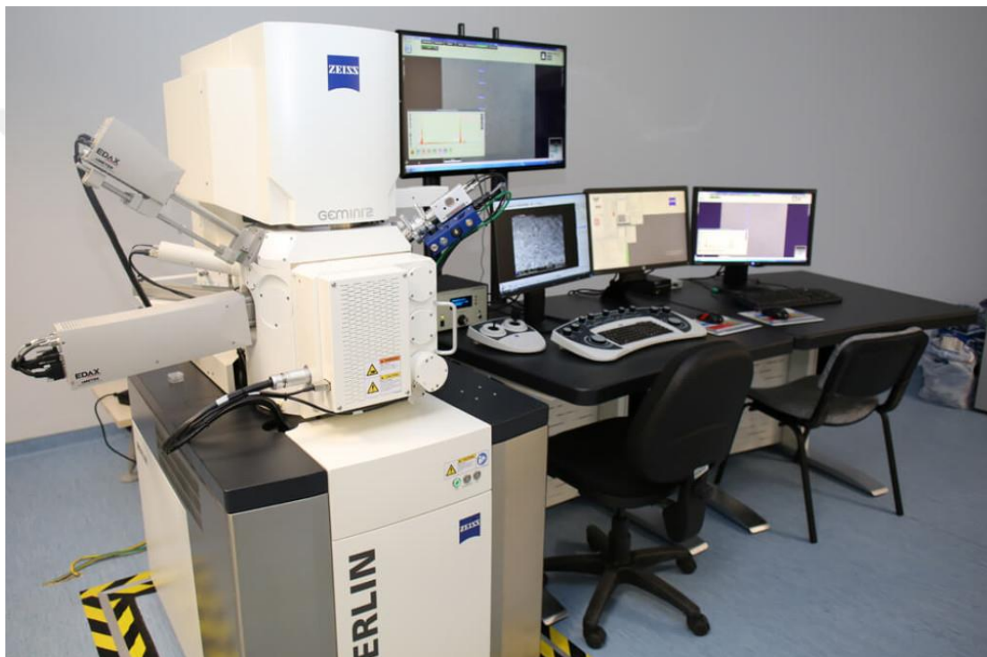
Figure 3.8 ZEISS MERLIN Scanning Electron Microscopy [32]
