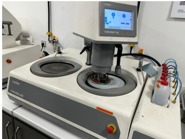
Figure 3.7 Metkon FORCIPOL 202 automatic grinding and polishing device [31]
