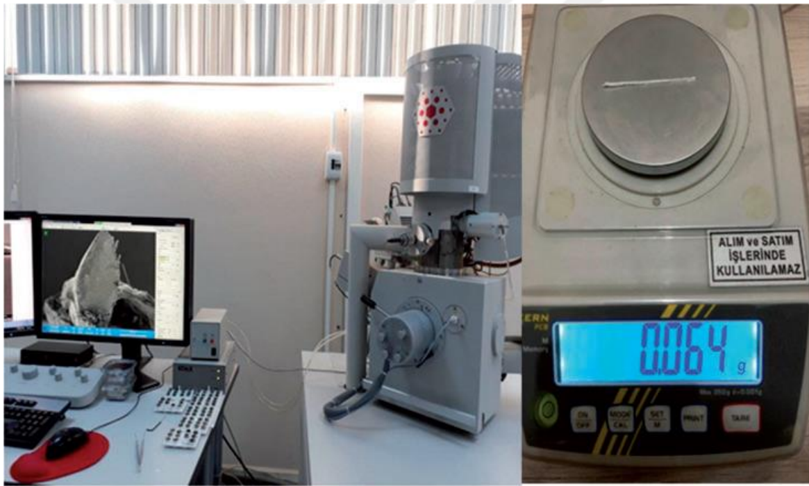
Figure 2.37 SEM device and weighing device [243].
