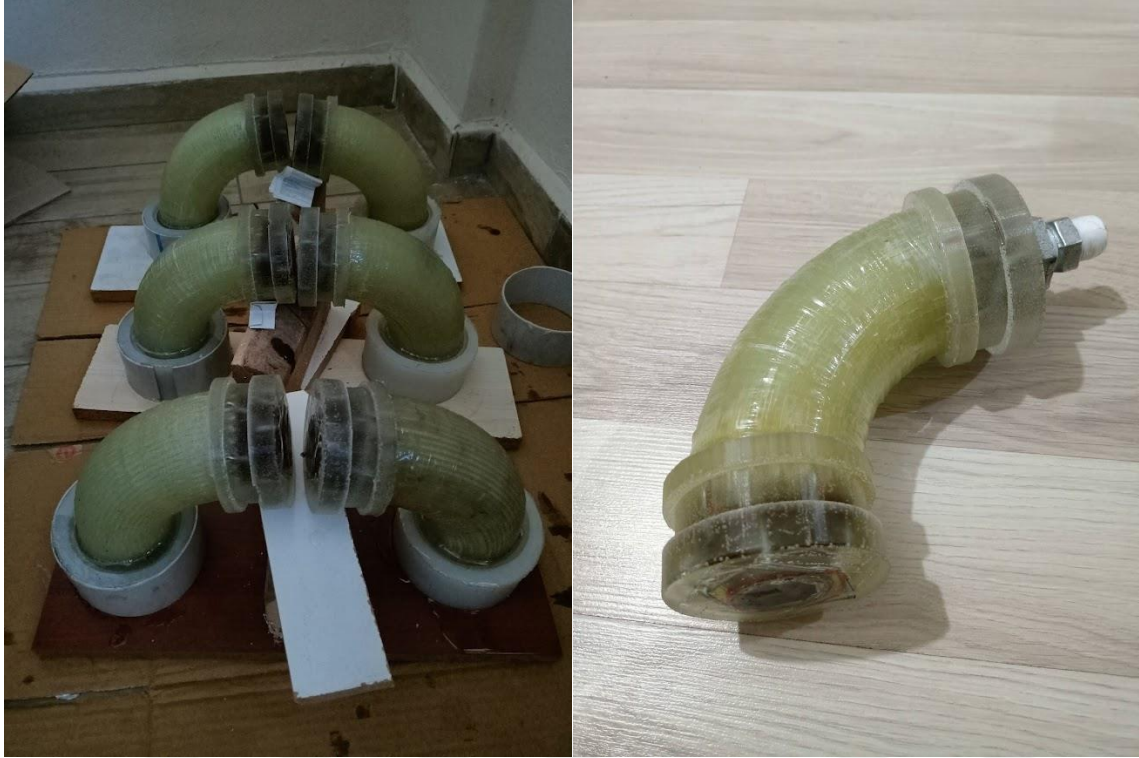
Figure 2.63 Composite elbow fitted with sealed and fluid fittings.
