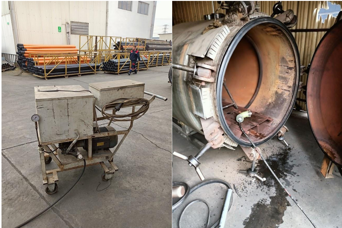
Figure 2.64 Application of internal pressure strength test to composite elbows.
