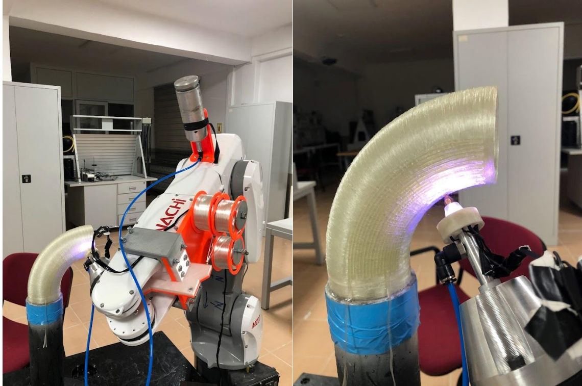
Figure 2.56 RAM with 75% filling rate in straight winding.
