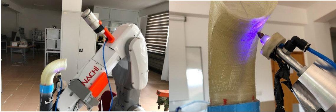
Figure 2.58 75% filling rate with the 1/8 turn angled helical winding.
