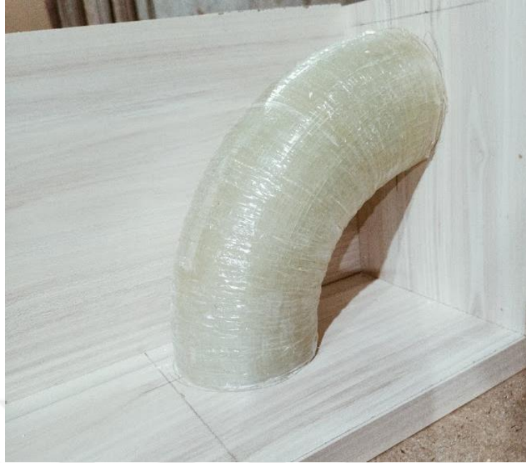
Figure 2.61 Cutting excess 90° composite elbow.
