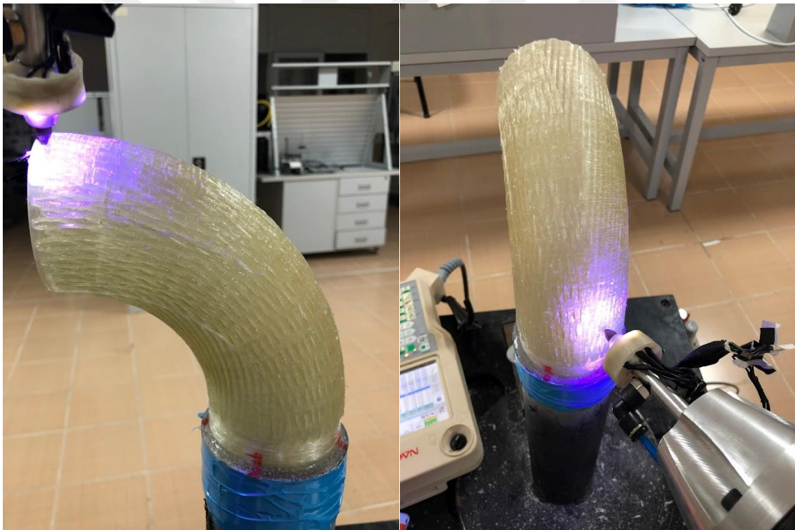
Figure 2.59 Winding of the reverse angled third layer.
