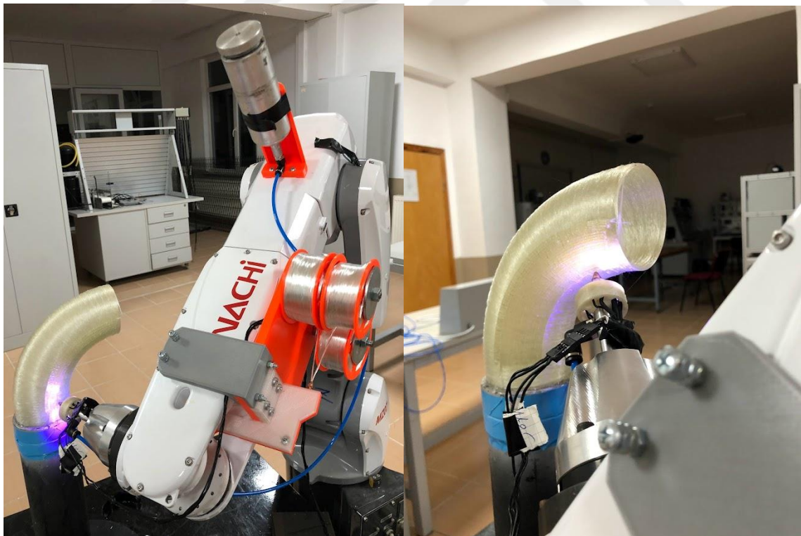
Figure 2.54 Straight fiber winding for the second layer.
