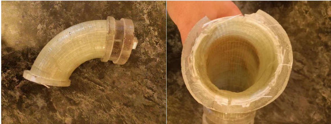
Figure 3.13 Image of the elbow after internal pressure test.
