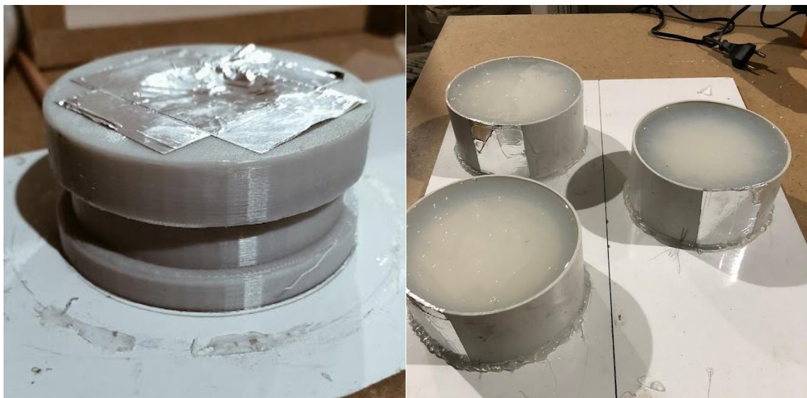
Figure 2.62 3D printed master model part and silicone mold casting.
