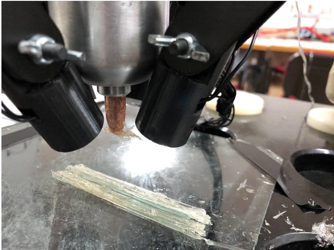
Figure 3.3 Production with lower fiber density which creates uncontrolled resin flow in RAM process.
