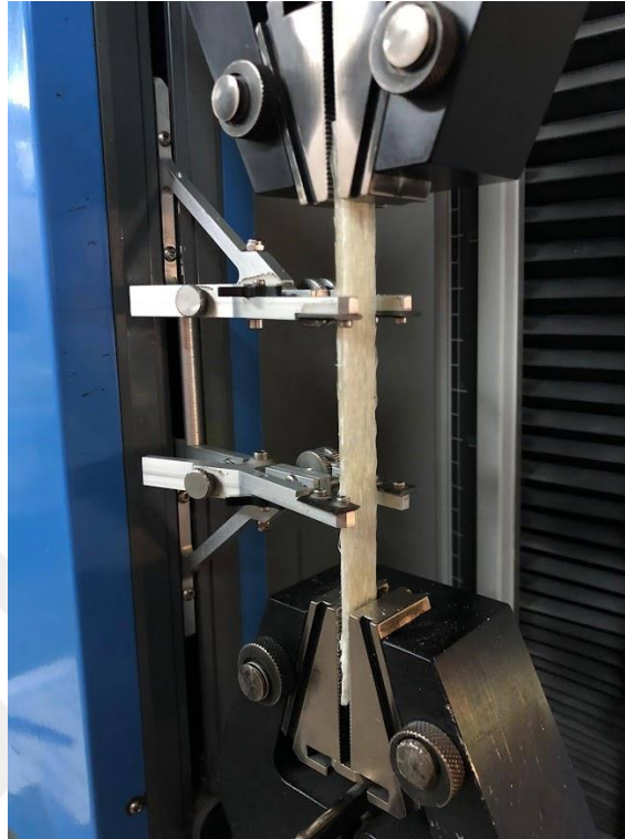
Figure 2.45 Tensile test process.
