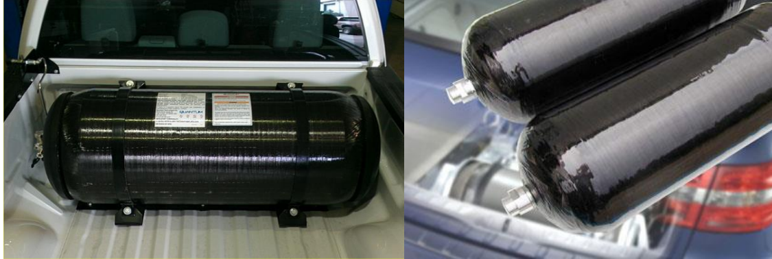
Figure 1.11 Vehicle Gas Tank (Left) Hydrogen Fuel Tube (Right) Fiber winding method in composite production [107, 108].
