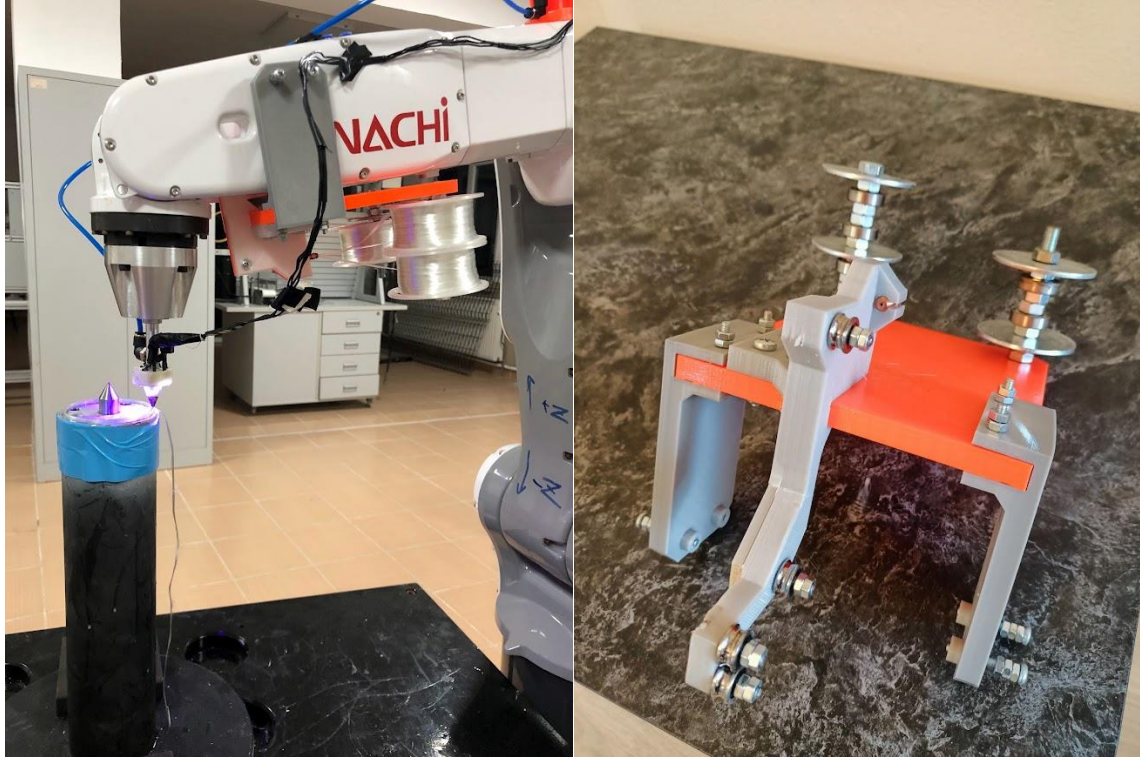
Figure 2.16 Final version of the revised tool for composite elbow production.
