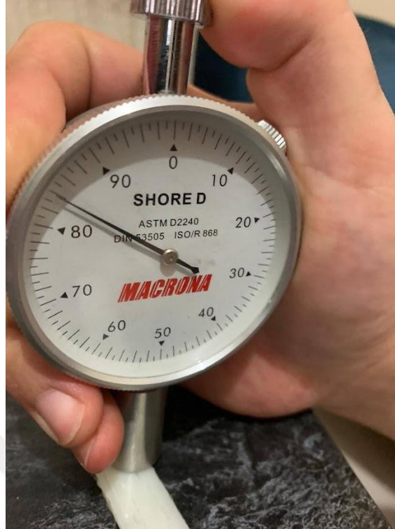
Figure 2.48 Shore D hardness test process.
