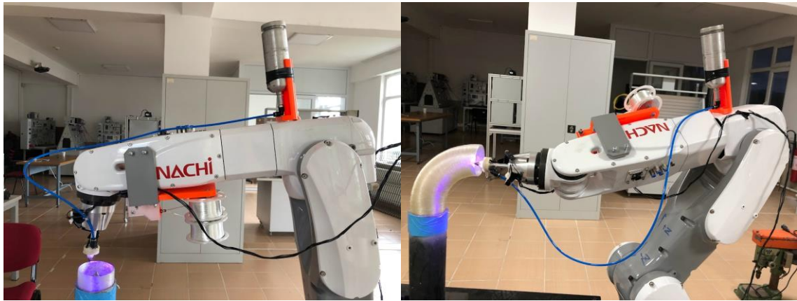
Figure 2.53 Production of the first layer of the 90° composite elbow.
