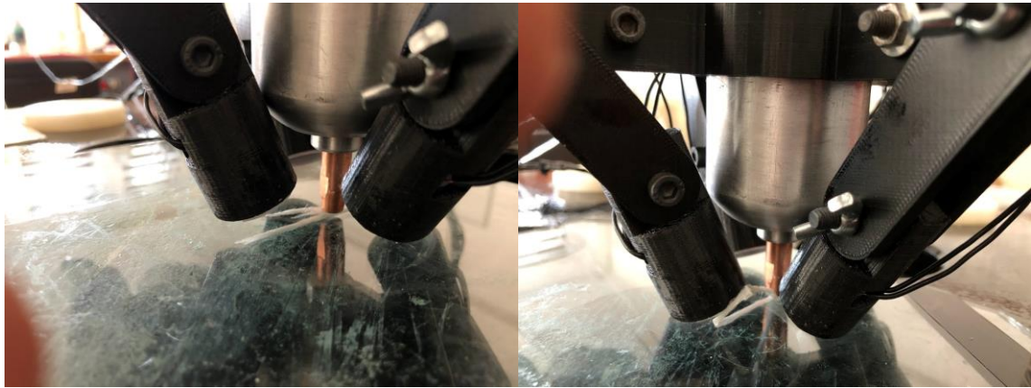
Figure 3.1 Fiber break and fiber retraction errors at corners.
