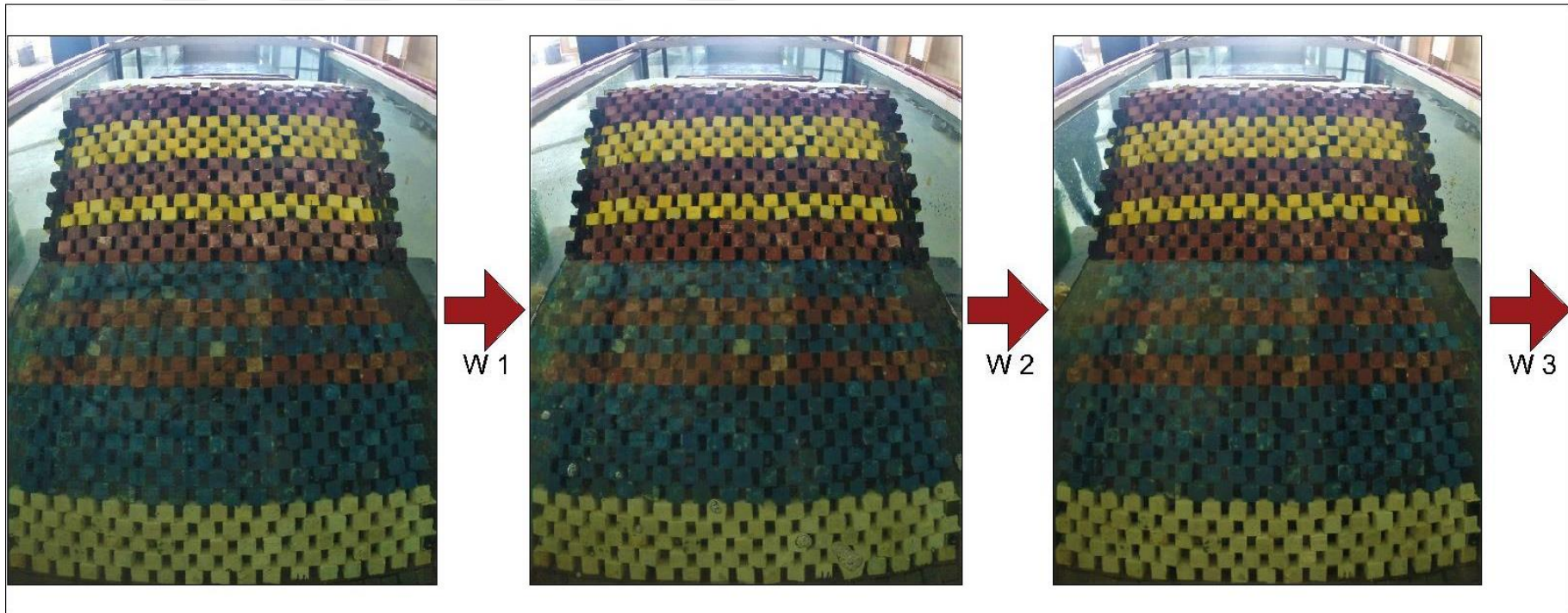
Figure B-11 Movement process (1) for Experiment 3: Single Layer HD Cubes with Regular Placement (no damage)
