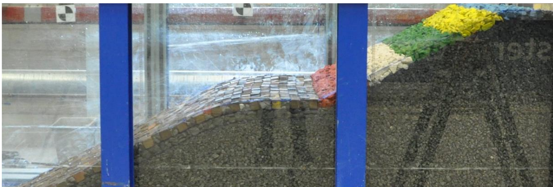
Figure 1.39 Physical model of the berm breakwater with single layer cubes (Van Gent and Van der Werf 2017)
