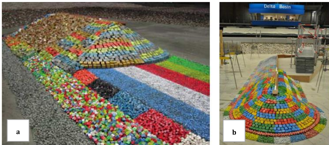
Figure 1.23 Model tests of single layer cubes for Punta Langosteira at left (a) and Boa Vista at right (b) (Van Gent and Luis 2013)
