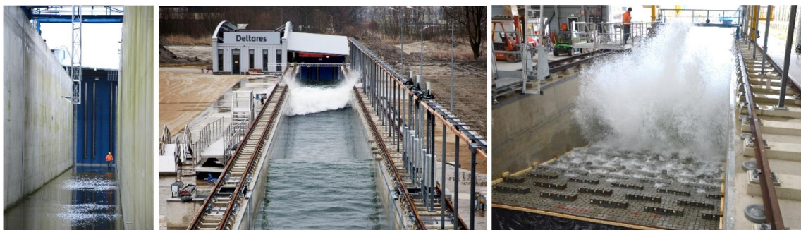
Figure 1.4 Flume tests of the Afsluitdijk at Deltares (Breteler et al. 2019)
