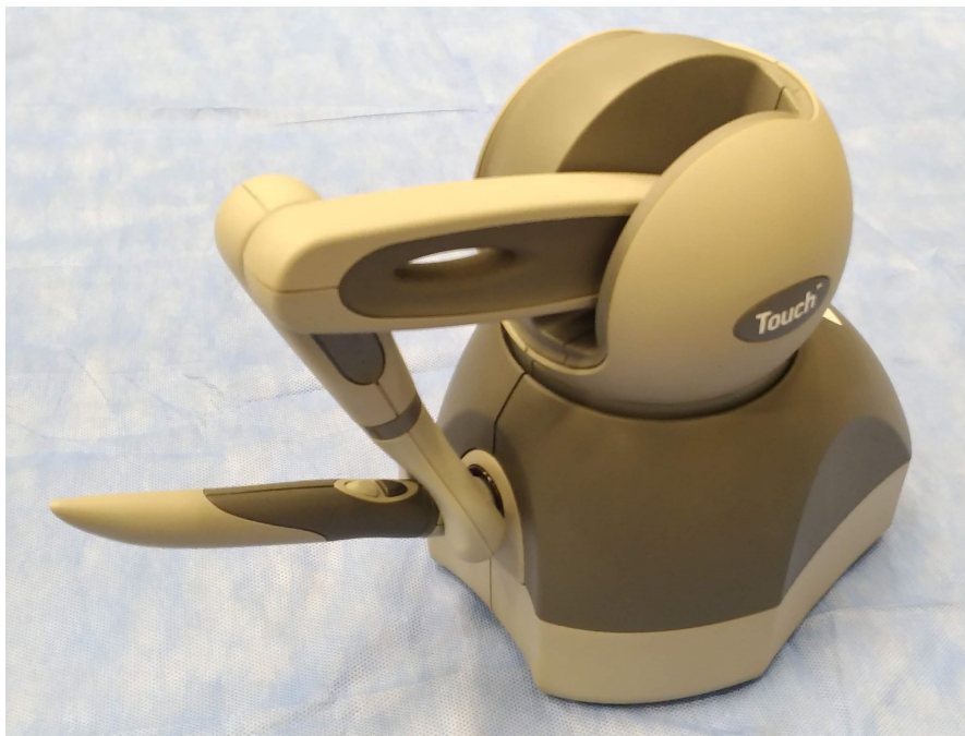
Figure 8: 3D Systems Touch haptic device
