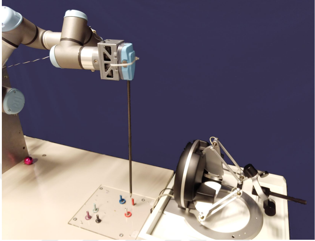
Figure 19: Experimental setup: 9-DOF surgical robotic arm, 6-DOF haptic device, and the task given to the subjects
