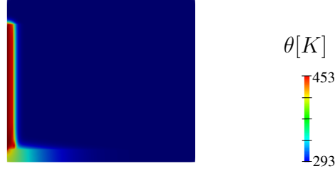
Figure 3.1: The simulation of the carbon fiber reinforced composite frontally cured
