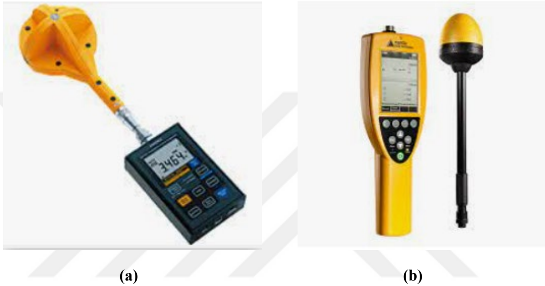
Şekil 3.6. a) HIOKI 3470 Magnetic Field Hitester; b) Narda Broadband Field Meter NBM-550
