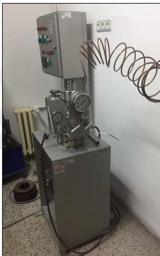
Figure 3.5 The lab-scale autoclave used in the carbonation experiments
