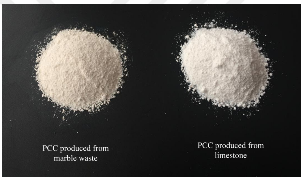
Figure 4.17 Produced PCCs from marble waste and limestone origin
