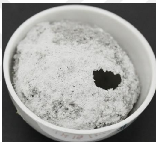
Figure 4.27 : Carbon char creation of PP70/IFR22/M6/C2 sample.
