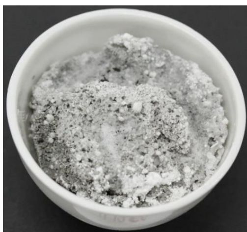
Figure 4.28 : Carbon char creation of PP70/IFR22/EG6/C2 sample.
