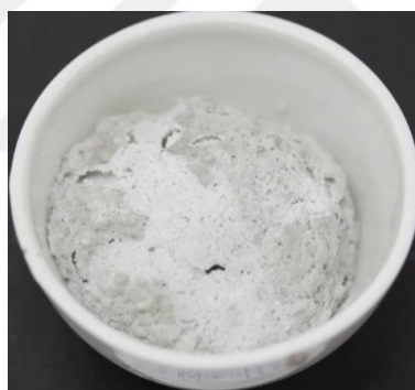
Figure 4.23 : Carbon char creation of IFR and colemanite.
