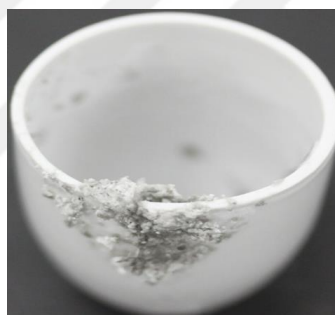
Figure 4.2 : Char residue picture after ash testing.
