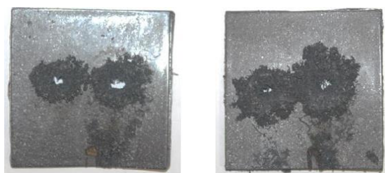
Figure 4.15 : Char forming on polypropylene surface during glow wire test.
