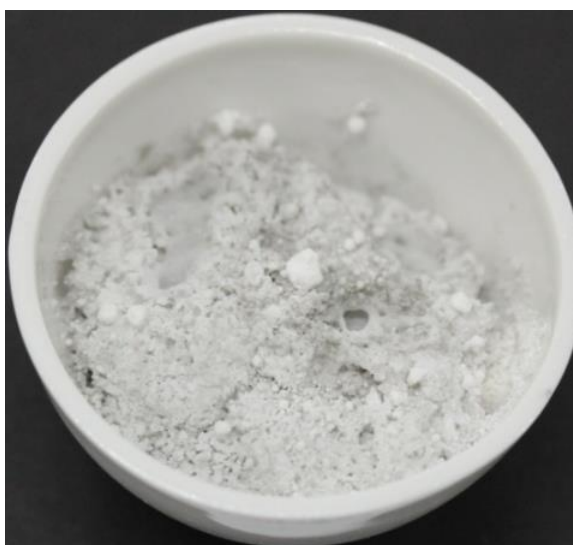
Figure 4.12 : The ash testing for PP70/IFR24/M6 sample.
