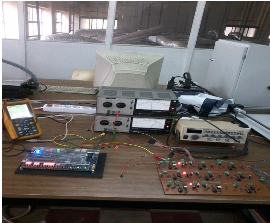
Figure 6.13 FPGA and interface circuit
