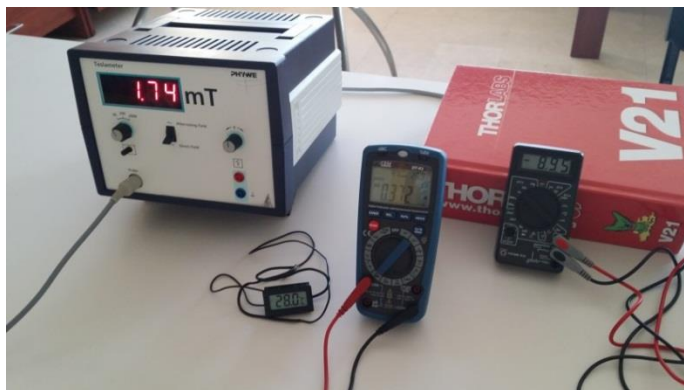
Figure 4.9 B-field, Temperature, Current and Voltage data taking set.
