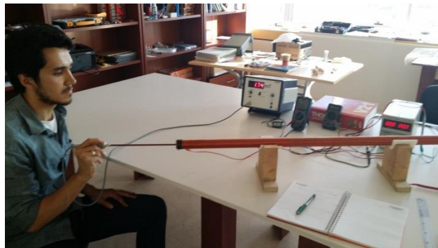
Figure 4.8 Taking magnetic field data from a depth within the solenoid.
