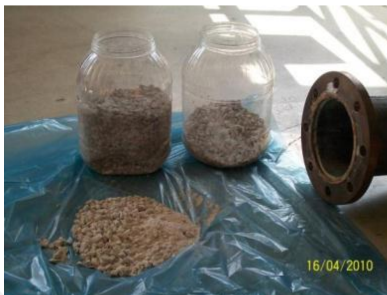
Figure 4.8. Used dolomite in the column.
