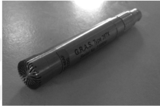
Figure 4.11. GRAS 46AF 1/2" LEMO Free-field Standard Microphone Set
