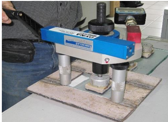
Figure 3.10: Test set-up of the adhesion test
