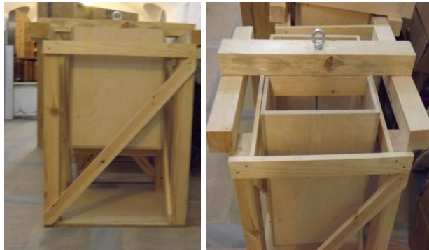
Figure 3.32: Loading box details of medium size specimen tests
