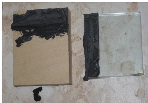
Figure 3.17: Mixed breakage-failure in adhesion to timber and cohesive failure in adhesive (laboratory conditions)
