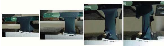
Figure 2.39: Elastic adhesives for timber-glass composites [30]
