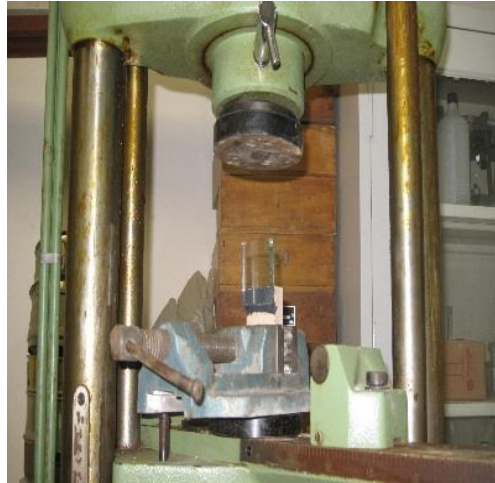
Figure 3.7: Loading device for shear tests
