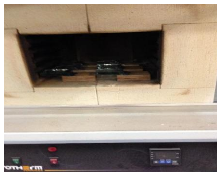
Figure 3.26: Timber-glass shear specimens after high temperature test
