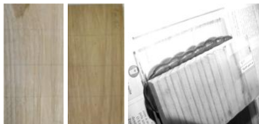
Figure 2.38a, b and c: Effects of solar radiation on timber surface with different colours - picture before (a) and after solar exposure (b) and on initially transparent adhesive (c) [29]
