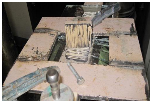
Figure 3.21: Failure in adhesion to timber cohesive failure in timber (laboratory conditions)
