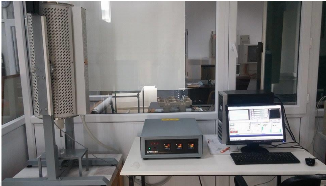
Figure 5.5. Dip coating measurement system for nano thin film
