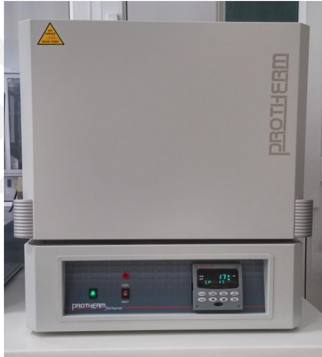
Figure 5.4. The high temperature muffle furnace
