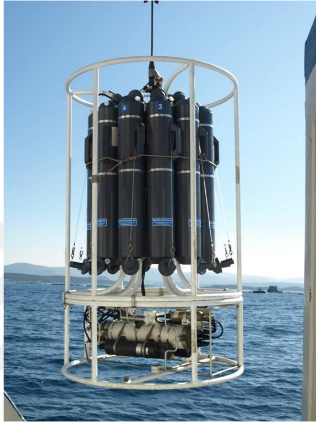
Figure 2.3 SBE 19plus V2 (Version 2) Seacat Profiler CTD on RV/K Piri Reis.
