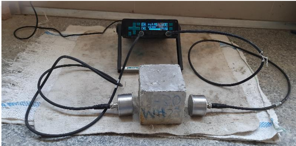
Figure 3. 13 Ultrasonic pulse velocity meter
