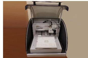
9) LPKF Circuit Board Plotter ProtoMat S63
