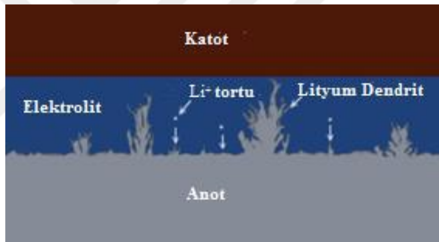
Figure 4.26. Schematic structure of Lithium dendrite growth [15].
