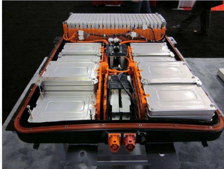
Figure 3.7. Li-Ion battery assembly (horizontal) [19].
