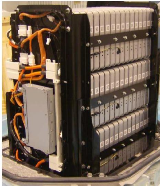
Figure 3.5. Li-Ion battery assembly (vertical) [19].
