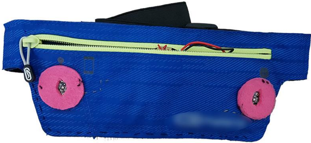
Figure 4.21 Interactive belt v1 (The sensors were framed but not covered)
