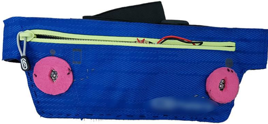
Figure 4.8 The first version of the interactive belt (Front view)
