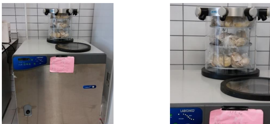
Figure 3.1. Lyophilizer (Left); Sliced tuber samples for lyophilization or Freeze drying (Right)
