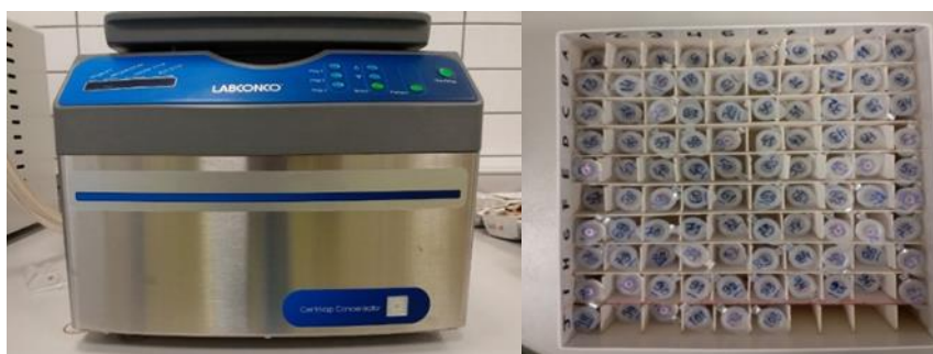
Figure 3.13. Centrivap Concentrator for drying DNA samples (a); Arrangement of Eppendorf tubes in a box containing 500ng of DNA in a dried form (b)
