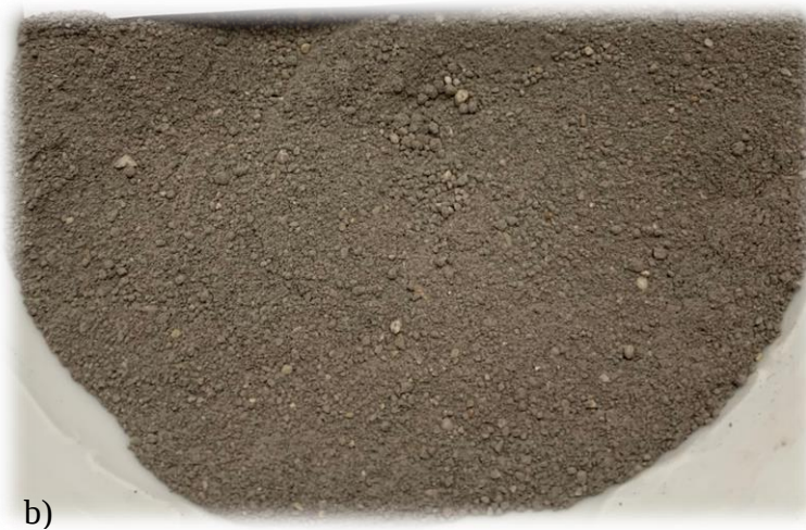
Figure 3.6 : Sile Sand 20/30 with a) 15% TT silt b) 25% TT silt used in this experimental program
