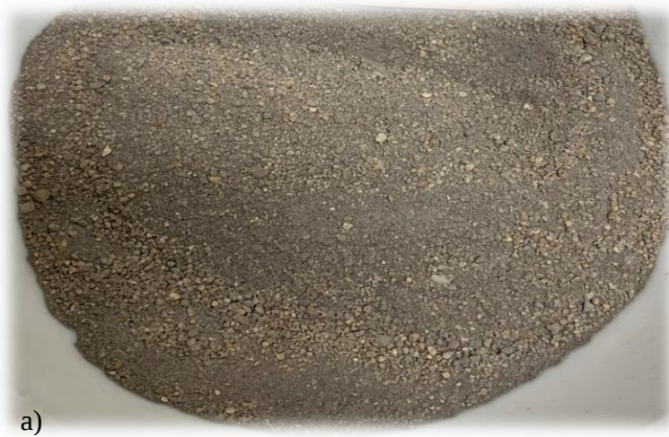
Figure 3.5 : Sile Sand 20/30 with a)15% IZ silt b) 20% IZ silt used in this experimental program
