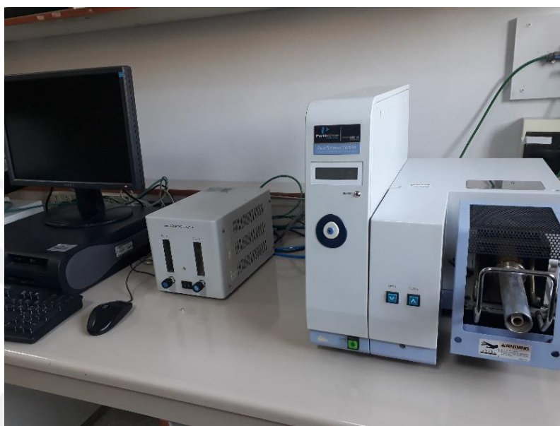
Figure 5.12. The TG/DTA device used for isothermal oxidation measurements of the NiTiSn-wire sample
