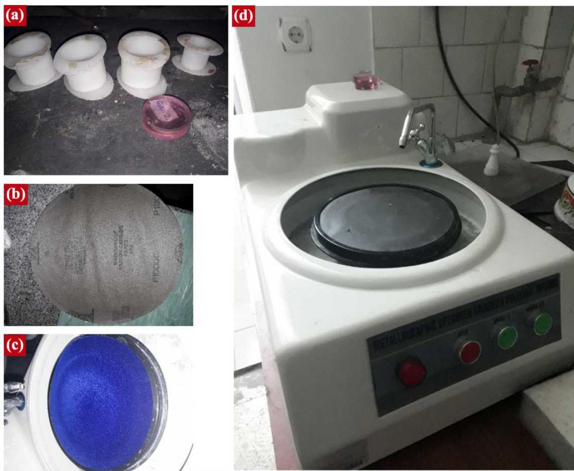
Figure 5.14. (a) Reusable plastic mold and a mounting example; (b) an emery paper; (c) polishing cloth; (d) metallographic sample grinder polisher machine
