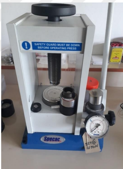
Figure 5.3. A manual compressor is used to pelletize the powders into a single pellet
