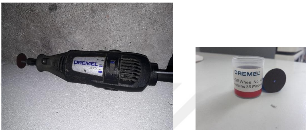
Figure 5.10. Electric Mini Grinder/Micro Drill, DREMEL ( left ), and Emery Cutting Disc ( right )
