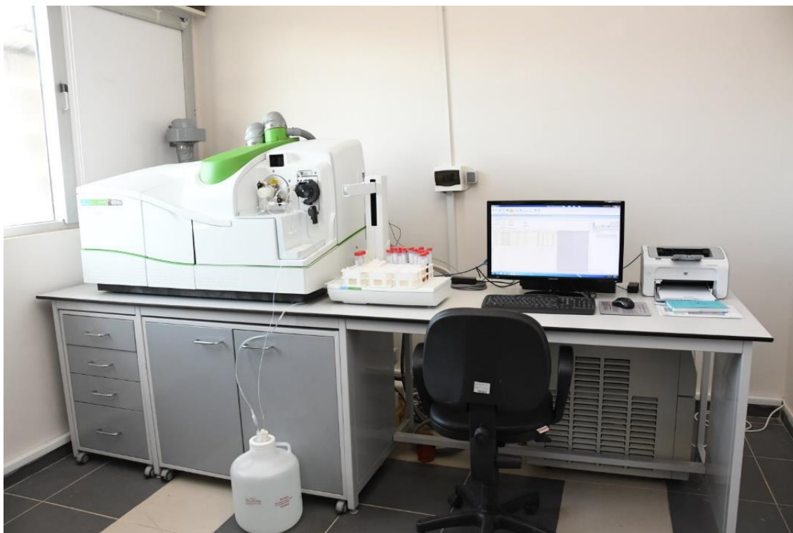
Figure 5.17. The ICP-MS is used for measuring the concentration rate of elements in SBF and PS.
