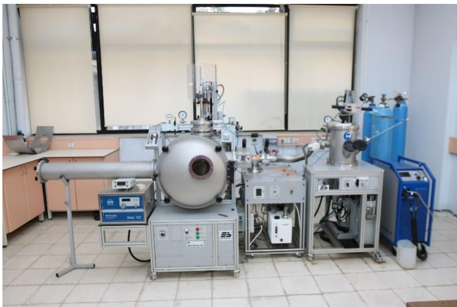
Figure 5.4 The Arc-melting furnace with a high vacuuming chamber and atmosphere control system
