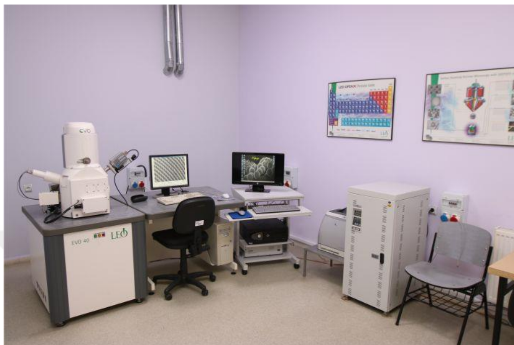
Figure 5.15. Scanning Electron Microscopy-Energy Dispersive X-ray Spectrometry (SEM-EDX) used for the morphology of microstructures and their chemical compositions
