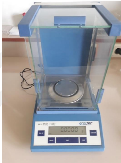
Figure 5.2. A sensitive digital balance that used to weigh the powders with an accuracy of 1mg
