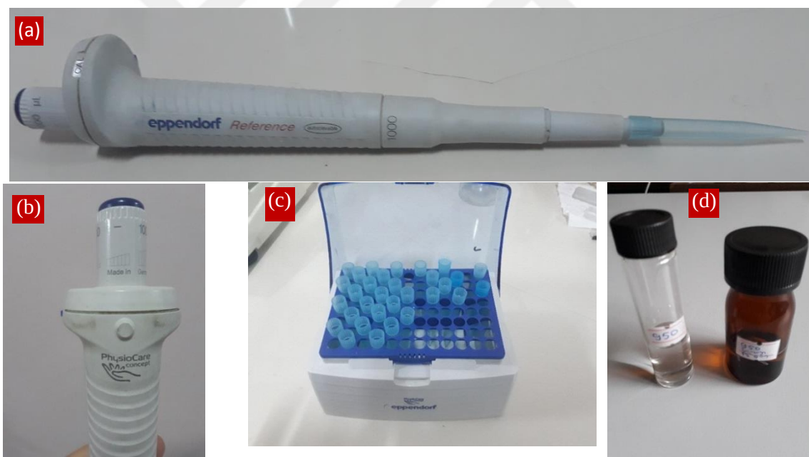
Figure 5.7. (a) A general view of a Lab pipette (Eppendorf Reference "Autoclavable" VARIABLE PIPETTE 100 - 1000 \mu l). (b) The front view of the pipette. (c) The pipette tips. (d) Bottles for an in-vitro test
