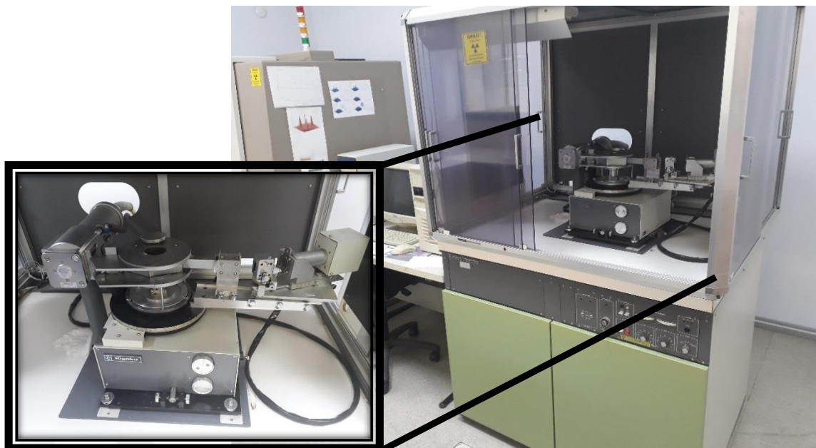
Figure 5.13. XRD device used for determining crystal structures of the samples
