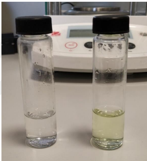
Figure 2.8: Spectrophotometric silicomolybdate method for \text{SiO}_{2(\text{aq})} analysis. Green color refers presence of \text{SiO}_{2(\text{aq})} in the solution.
