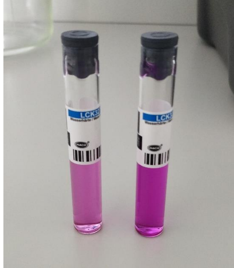
Figure 2.9: Spectrophotometric measurements for Ca and Mg in the solution.
