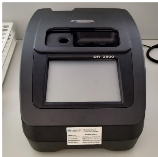
Figure 2.6: Hach Lange DR 2800 Spectrophotometer.
