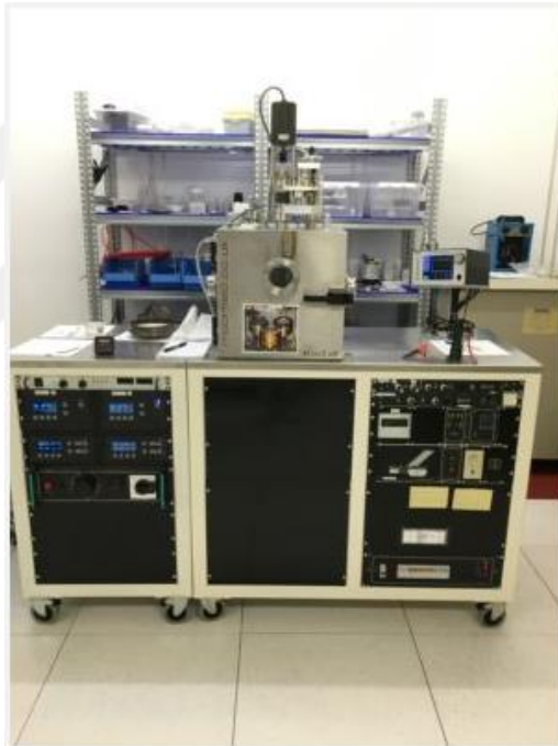
Figure 3.17 Moorfield - DC/RF Magnetron sputtering set-up.
