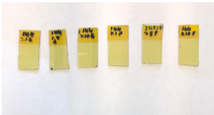
Figure 3.10 PVB and PVP encapsulated YHO films.
