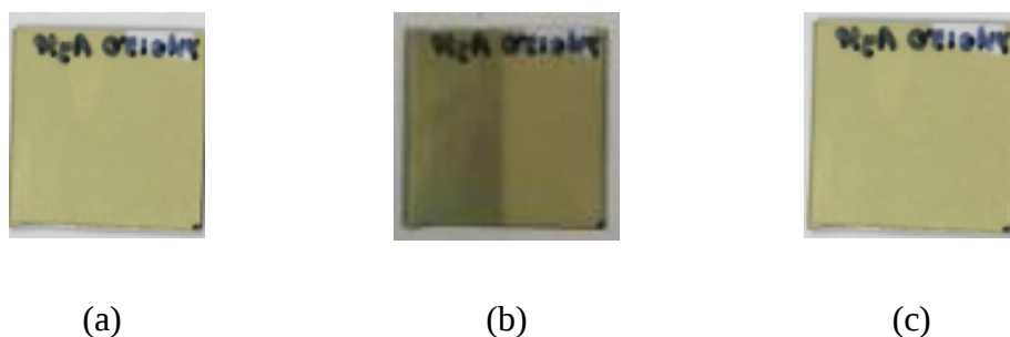
Figure 3.7 \text{Al}_2\text{O}_3 encapsulated YHO films (a) As-deposited film (b) UV illumination film (c) bleached film.
