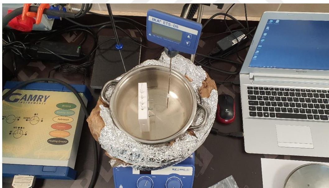
Figure 3.10: The cell placement in the pot.
