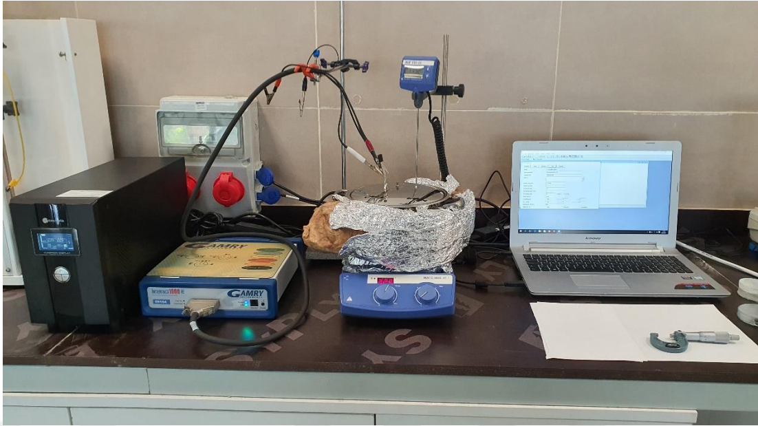
Figure 3.11: The experimental setup for the impedance measurements.
