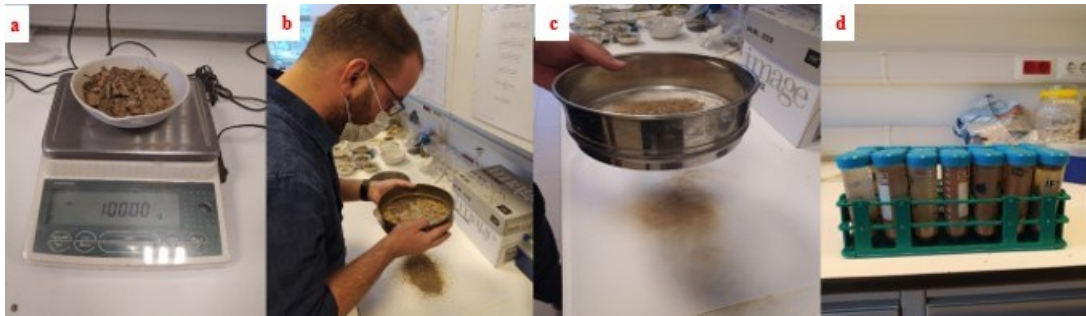
Figure 3.6: Laboratory analysis steps for soil texture analysis, a) weighing soil samples, b) sieve analysis for gravel and sand, c) sieve analysis for silt and clay, d) fine particle size collection for Mastersizer analysis.
