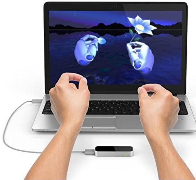
**Figure 2.29 :** LeapMotion controller connected to a laptop (Url-11).
