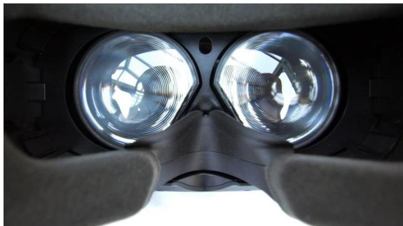
**Figure 2.27 :** Close-up of HTC Vive’s lenses (Image credit: Valve Corporation).
