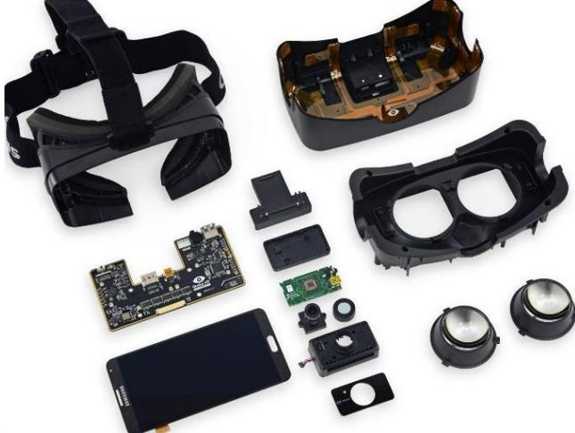
**Figure 2.11 :** Oculus Rift DK2 teardown (Image credit: iFixit Co., LTD.).
