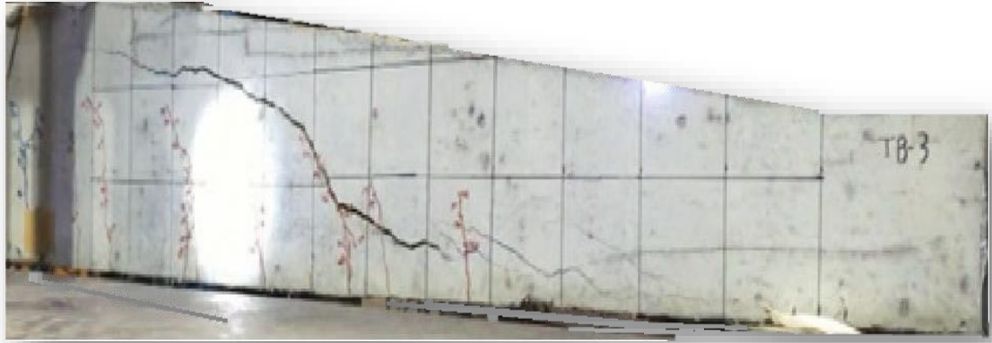
Figure 3.10 After peak of TB3-3 beam in EXP [1].
