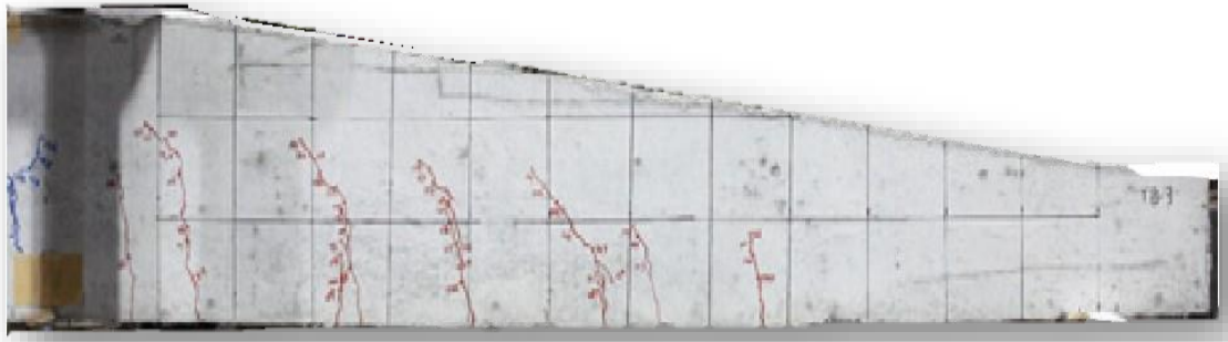
Figure 3.7 Just before peak of TB3-3 beam in EXP [1].
