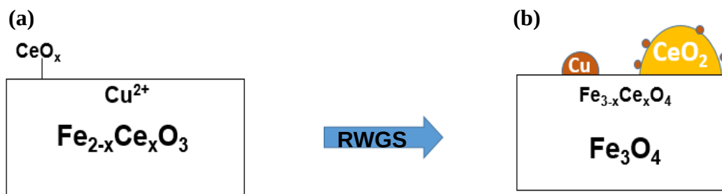
Figure 6.17. Schematic of the 3Cu/8CeFe catalyst (a) calcined and (b) during HT-WGS
