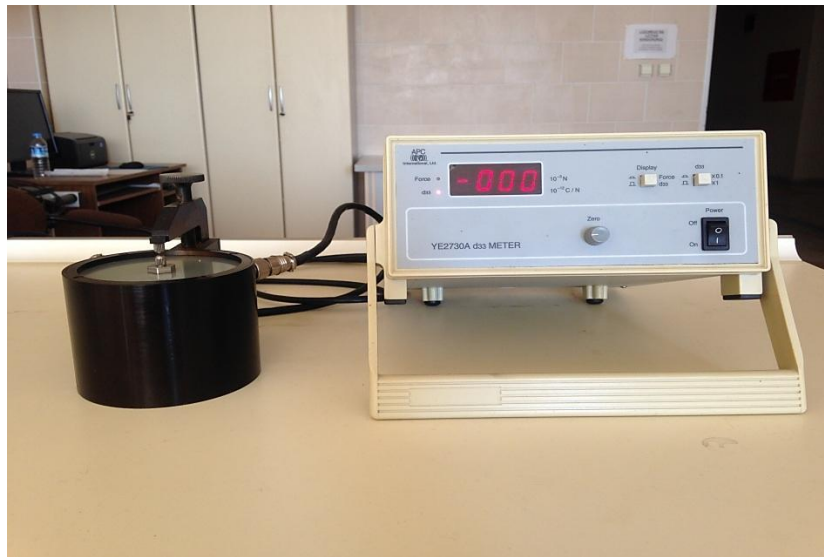
Resim 3.8 APC International YE2730A marka d_{33} metre.
