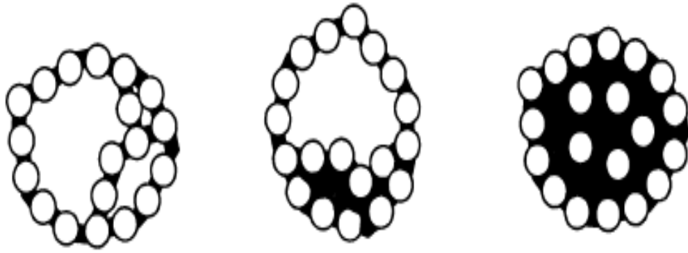
Figure 2.3 Mechanism of pellet formation during pelletization process (Jaroslav and Ruzickova, 1987)
