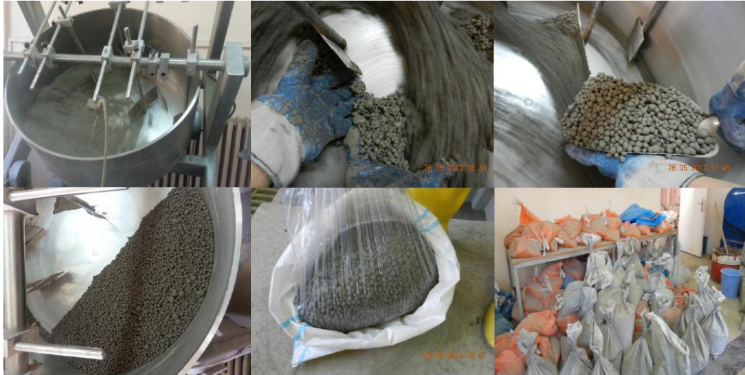
Figure 3.3 Production of artificial lightweight aggregate through cold bonded process
