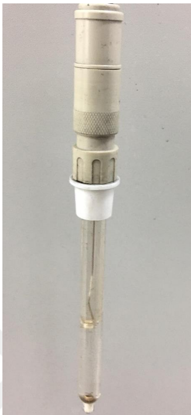
Figure 3.5 The image of double junction Ag/AgCl (saturated KCl) reference electrode
