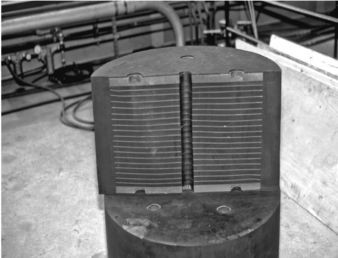
Figure 2.13 Typical of Natural rubber isolator (Tarics et al., 1984)
